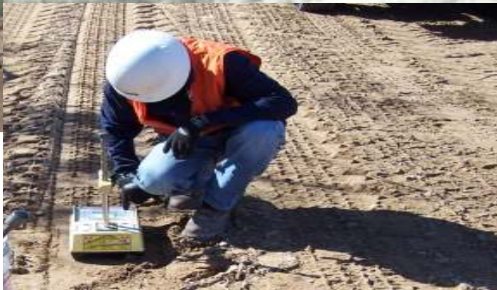
(on right) Compaction and density testing using Nuclear gauge method
