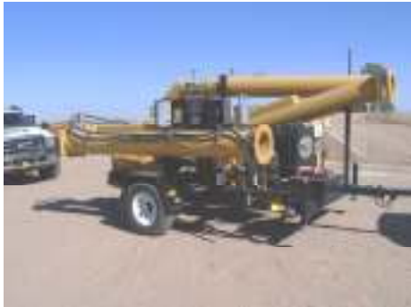
The pump (left) is a diesel operated 14” centrifugal single stage unit and was set into the Salinity Canal near the construction area on October 22, 2008. Water was delivered to the construction area using water trucks. (below) a water truck “filling up” at the pump
